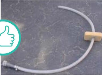
**HOSE HAS NO KINKS AND INCLUDES A SPONGE TO REDUCE LEAKAGE AT PENETRATION WHEN INSULATING**
