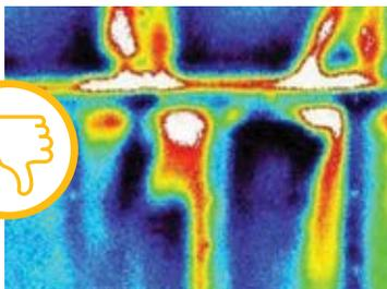
**INFRARED POORLY INSTALLED WALL INSULATION**
